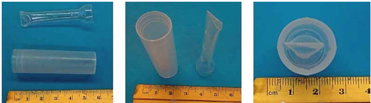
Figure 3: Thin-walled polyethylene vial with poly insert designed to disperse sample.
