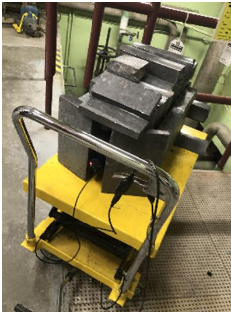
Figure 2 NaI detector shielded by lead
