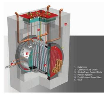
Figure 3: CANDU Reactor Core.
