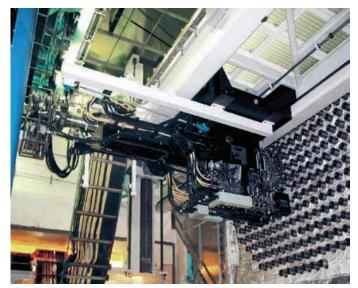
Figure 4: CANDU Reactor Fuelling Machine.
