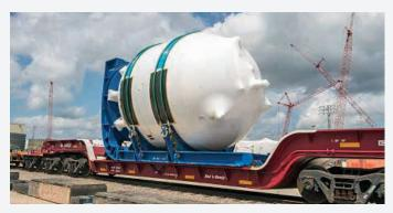
the steam generators were produced in South Korea. Overseas equipment is being delivered by rail from the port of Savannah.
