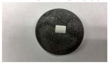
Figure 5 Zirconium specimen after polishing
