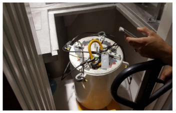
Figure 3 Vertical flask in receiving cell during cold commissioning
