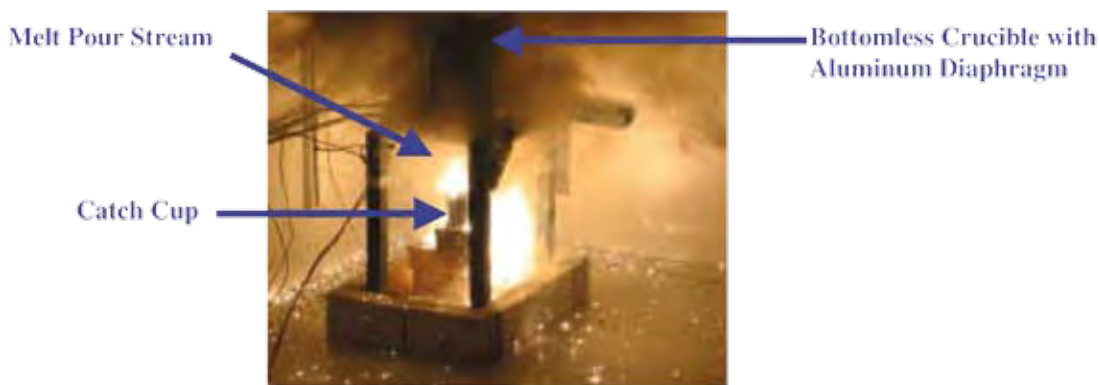
Figure 3: A photographic view of the melt-pour stream dripping out of the crucible.
