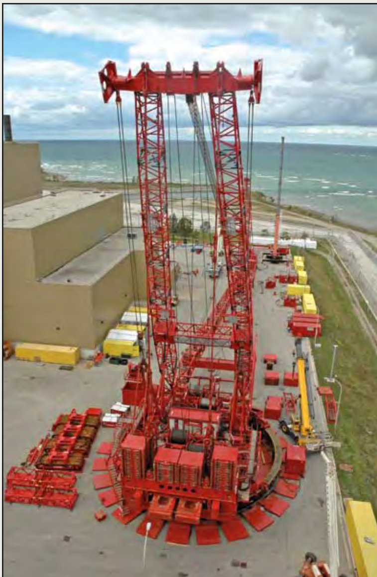
A view of the massive Mammoet crane to be used for the replacement of the steam generators.
