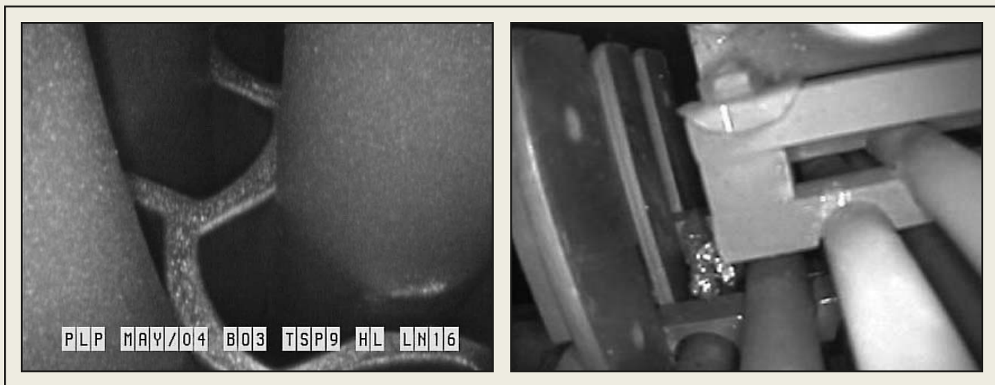
Figure 6: Visual Inspection Images Showing Lack of Fouling in the Upper Bundle. Left: hot leg broached holes in support 9 in steam generator 3 in 2004. Right: U-bend scallop bar supports in steam generator 4 in 2006
