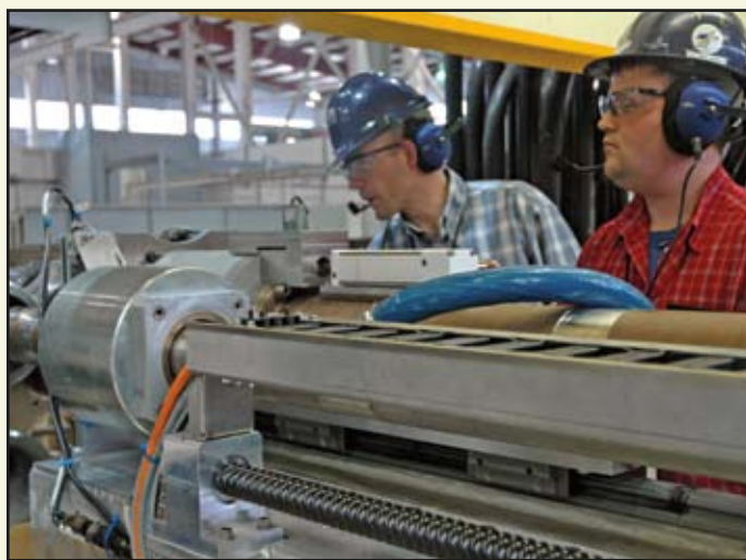
Electrical Engineer David McDonald and Electrician Joel Merswolke monitor a test of the Pressure Tube Severing Tool on a reactor mockup in Bruce Power's Technical Mockup Building.
