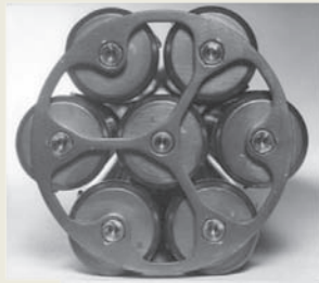
NPD 7-el bundle ~ 1955 - 8 cm Pressure Tube ID
