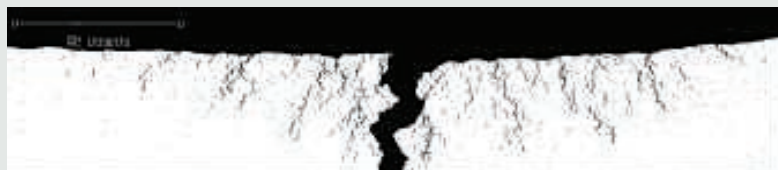
Optical micrograph of feeder S08a showing secondary cracking near the mouth of the main inside surface crack.
