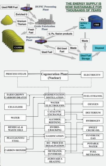
Figure 6 – Potential ladder of industrial processes at BNPD [15]
