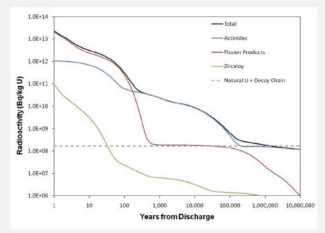
Figure 1: Activity Versus Time for CANDU Fuel with a 220 MWh/kgU Burnup
