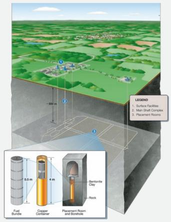
Figure 2: Conceptual Geological Repository With Vertical Placement
