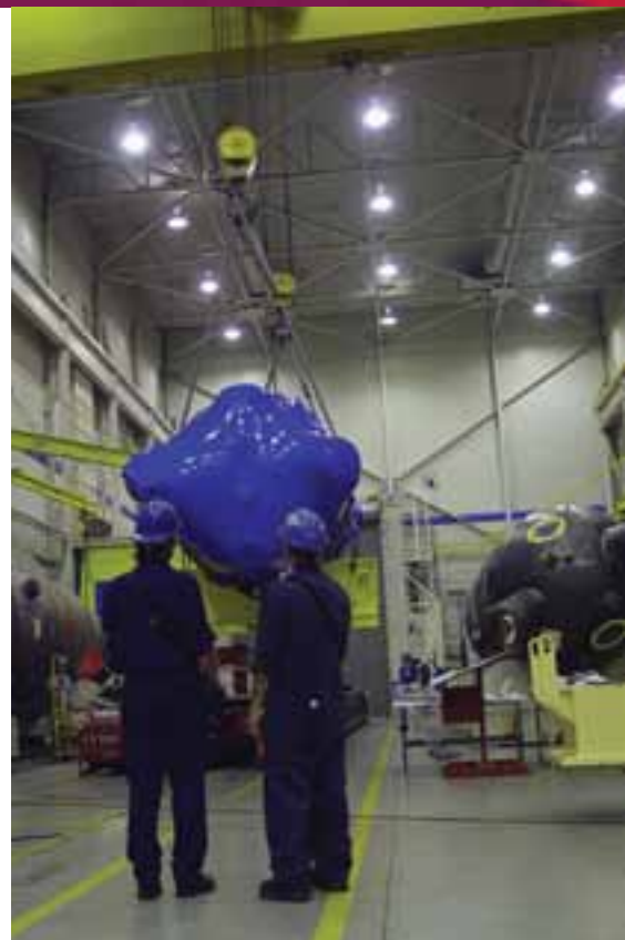
Steam generator packaging and shipment at the Cambridge plant of Babcock and Wilcox.
