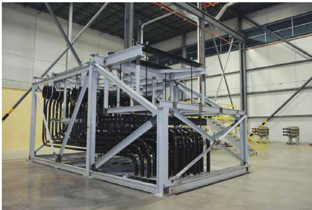
Floor mock-up with upper feeder pipe attachment to feeder cabinet header. (Photo courtesy of OPG)
