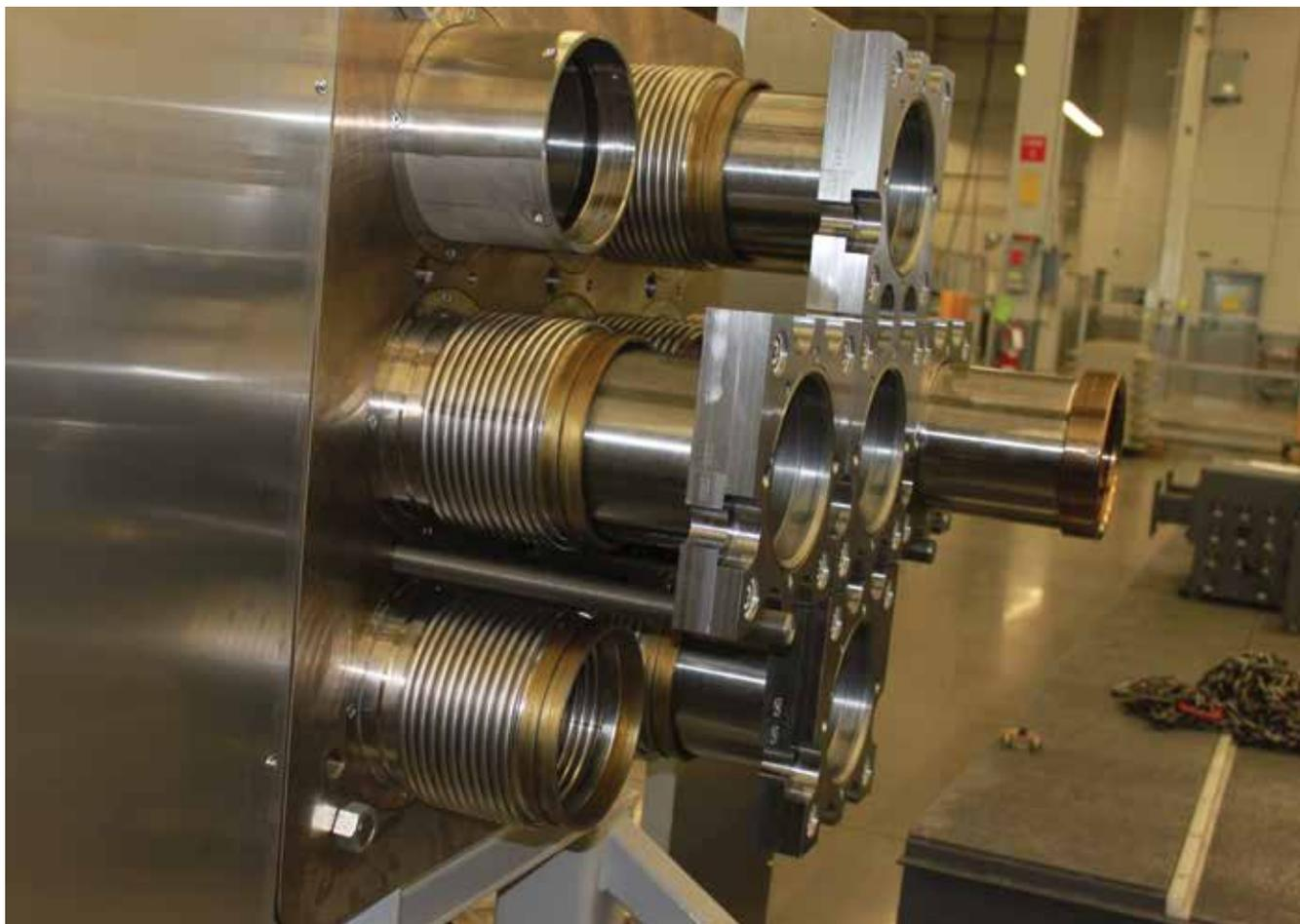
3 x 3 array floor mockup with bellows (intend to remove and reuse). (Photo courtesy of OPG)
