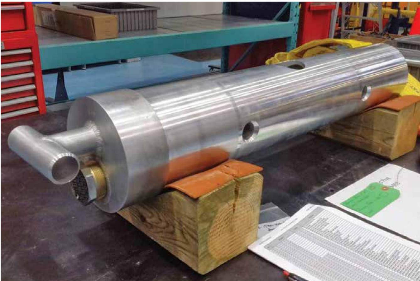
CV inspection – vented shield plug. (Photo courtesy of OPG)
