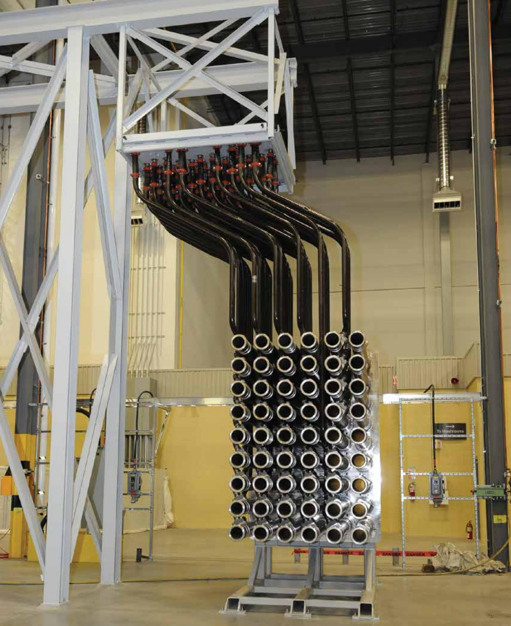
Floor mock-up 6 x 9 array with fuel channel tubes, end fittings and lower feeder pipes. (Photo courtesy of OPG)
