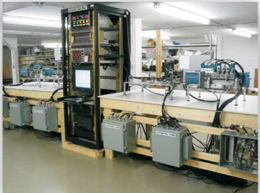
Failed Fuel Location / Delayed Neutron Detection System
