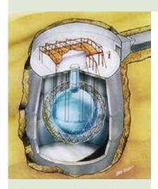
Above is a schematic diagram of the Sudbury Neutrino Observatory (SNO). It was located underground to eliminate interference by cosmic radiation. Its core was a 12-metre in diameter container filled with 1,000 tons of heavy water, surrounded by detectors.
