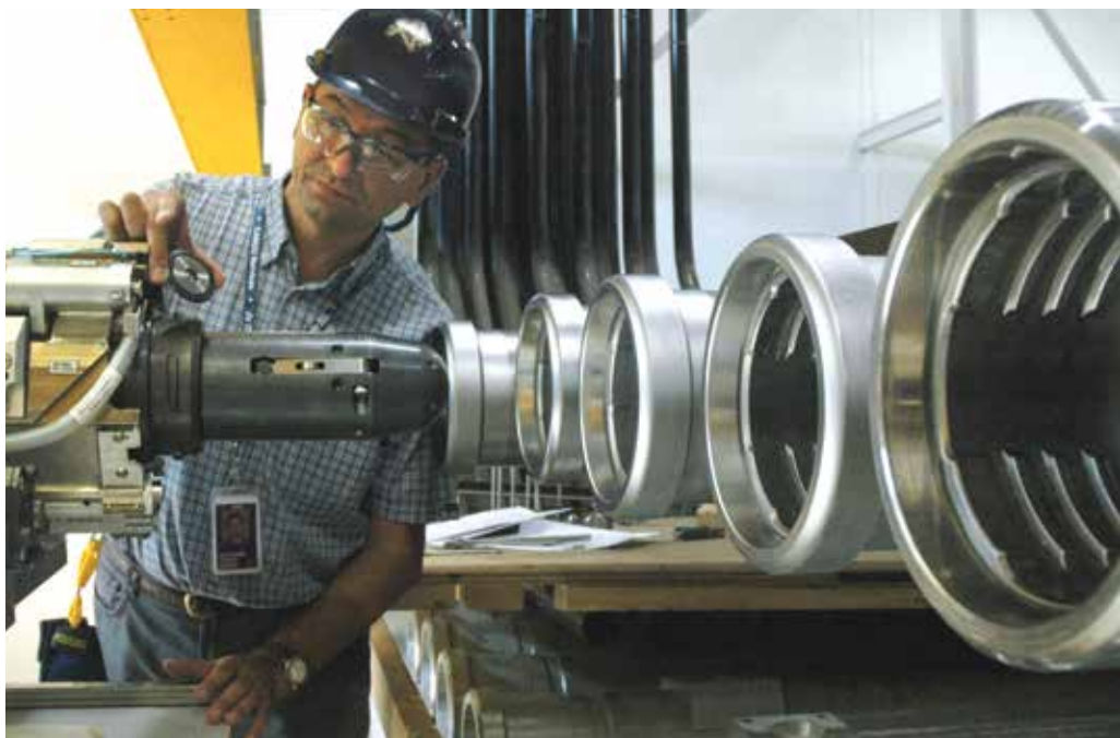
Preparing for fuel channel replacement. (Bruce Power photo)
