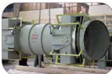
Main steam penetration gimbal expansion joints
