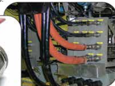
Thorburn quick couplings on a CANDU fueling machine
