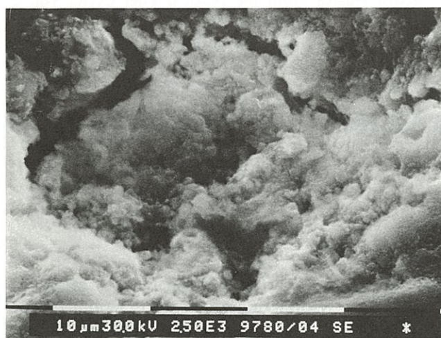
Figure 4: Inner pore space of a cementitious product; w/c ratio 0.34; \text{CsNO}_3 50 g/l.
