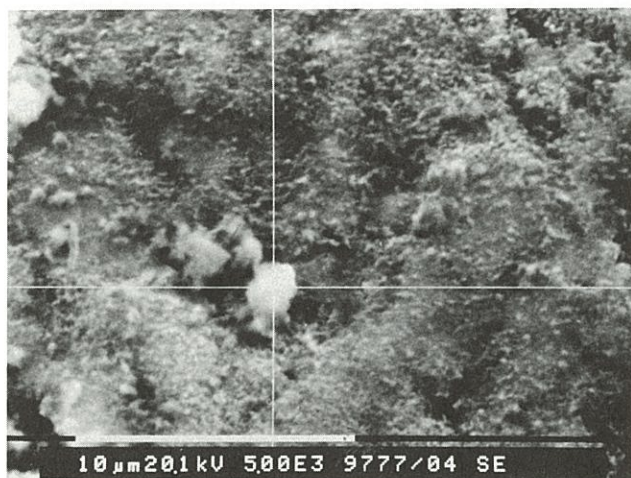
Figure 5: Globular \text{CsNO}_3 precipitation in the pore space matrix.
