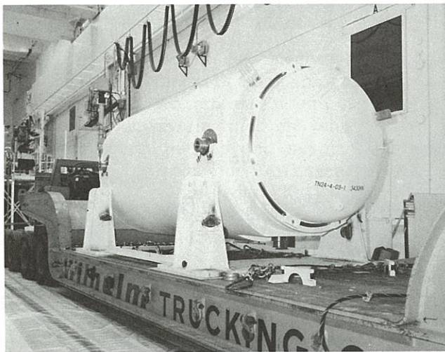
Figure 3: The second storage cask (TN-24P) built by Transnuclear, Inc.
