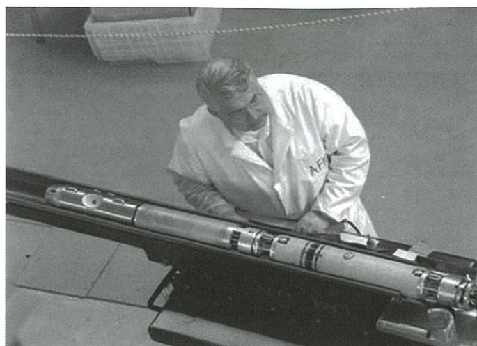
Figure 3: The NDE Head. The RIM is on the far left, the Motor Module in the centre, and the Sag Module on the right-hand-side.
