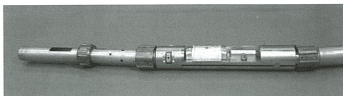
Figure 4: Re-Inspection Head. The Video Module on the left, the NDE Module in the centre, and the Replication Module on the right-hand-side.
