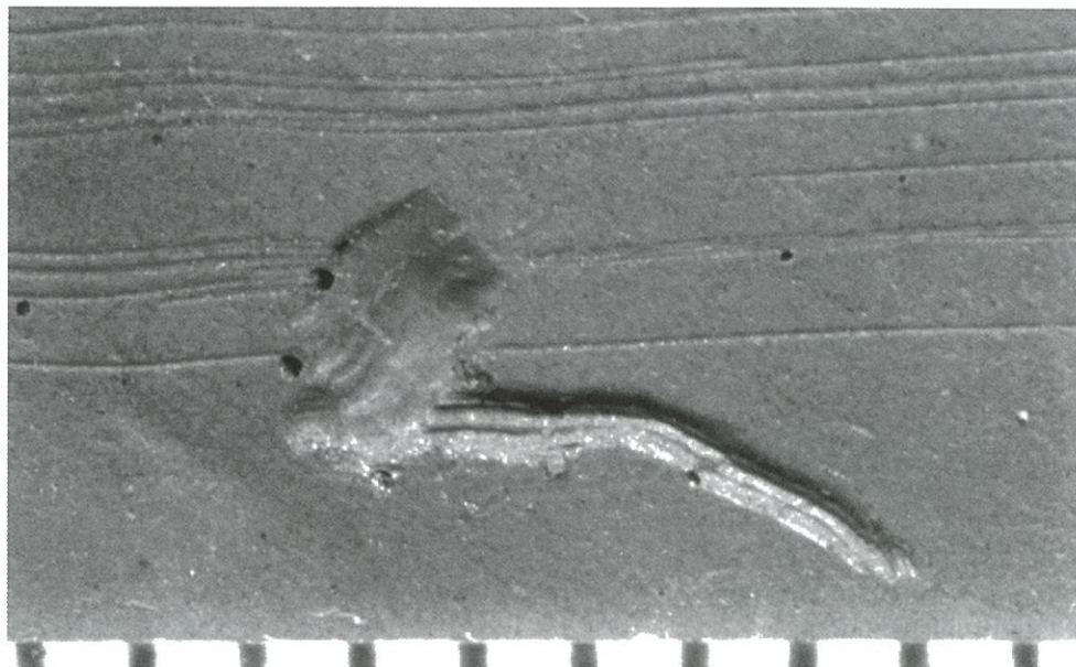
Figure 17: Macrophoto of a replica of a debris flaw obtained with AFCIS. The horizontal marks are fuelling tracks – they are slightly curved due to replica distortion. The flaw is about 6 mm long. The small circular objects are artifacts from debris or bubbles in the replicating compound.
