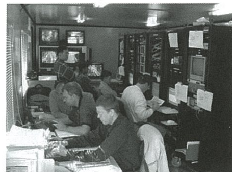
Figure 6: AFCIS data acquisition system. The six racks along the right-hand side of the figure are (from back to front): ADM control, SCADA, UT rack, ET rack, gauging rack, and re-inspection rack.
