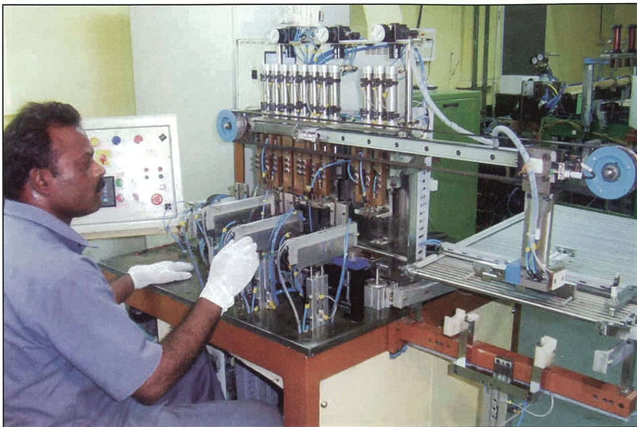
Fig 3: Integrated Spacer and Bearing Pad Welding Machine
