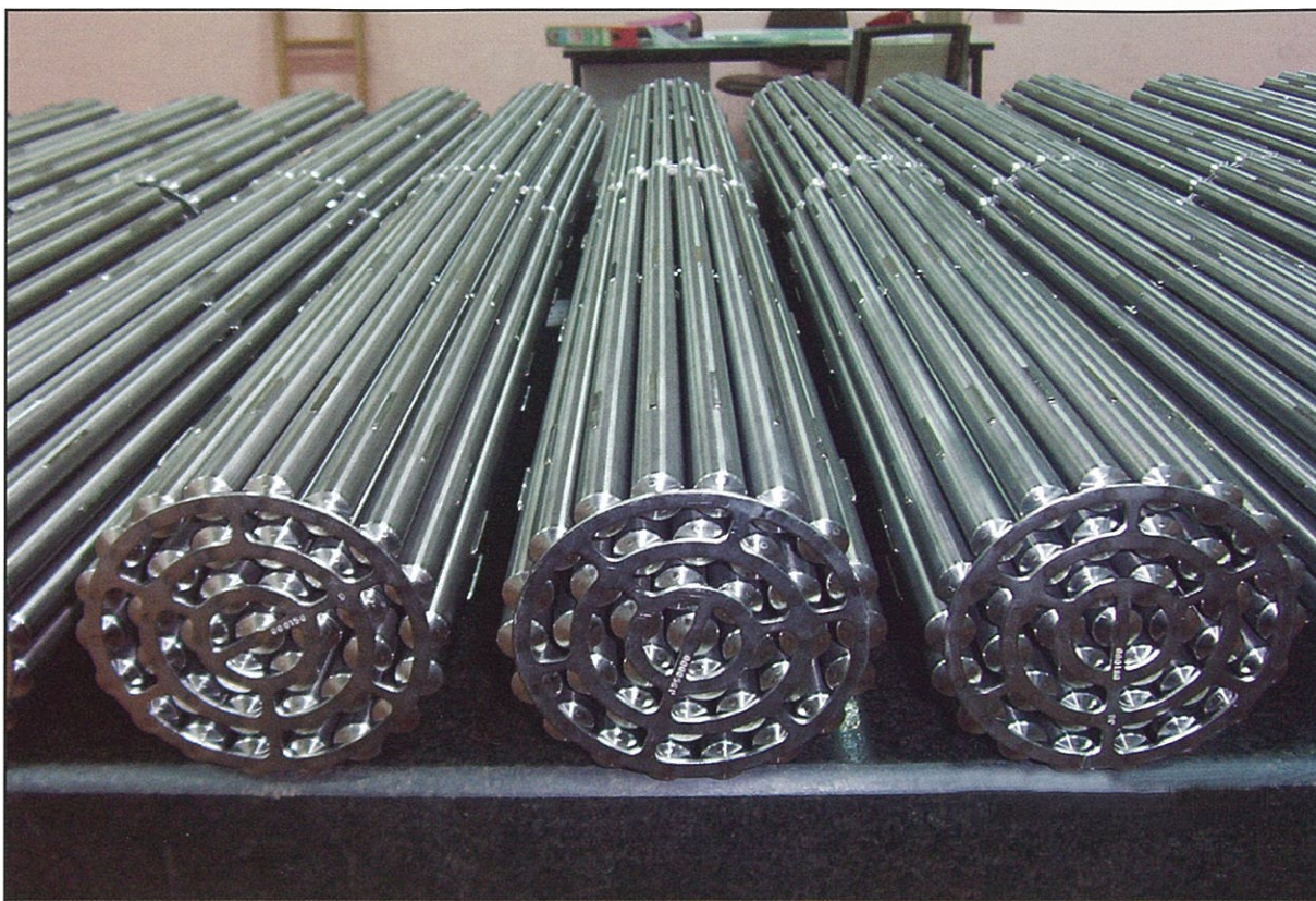
Figure 2: 37-Element Fuel Bundles for 540 MWe PHWRs.
