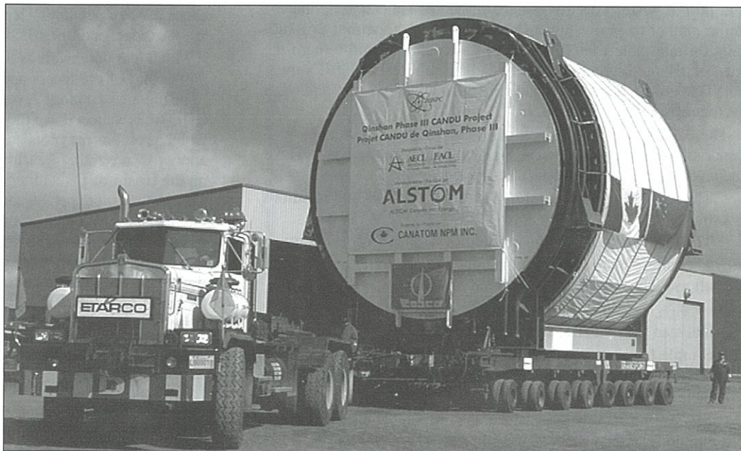
Tracy, Quebec: The first of two CANDU nuclear reactor cores for Qinshan, China, rolled out on April 15, 1999. The calandria, designed by Atomic Energy of Canada Ltd, was manufactured by Alstom Canada Inc. in Tracy, Quebec, under a subcontract to Canatom NPM, and will reach China in mid-June on a Chinese freighter. In total, the Qinshan project will result in $1.5 billion in revenue to Canadian private sector companies for goods and services, and 27,000 person-years of employment over the life of the project.
