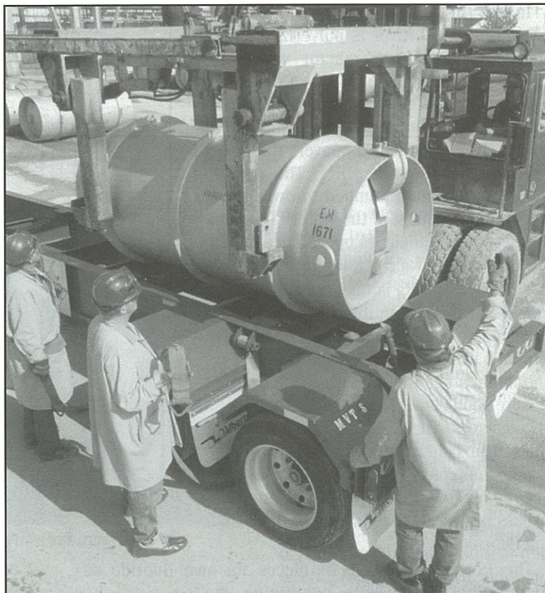
A UF_6 cylinder is placed on a trailer at the Port Hope conversion facility in preparation for the journey to an enrichment facility.
