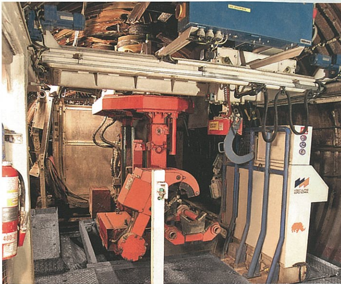
At Cigar Lake, the innovative jetboring mining method loosens the ore with jets of high-pressure water.
