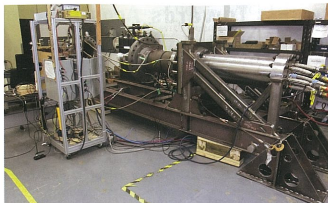
Figure 2: 'HP3b' acoustic driver test stand. The grey acoustic driver can be seen on the left hand side, while the large silver tube on the right, is an energy absorbing device used in place of liquid metal.
